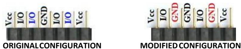
By having the highlighted I/O pin connected to GND the ground bounce can be improved by 42%.
